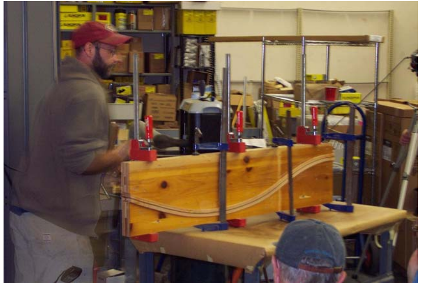
This is a clamping jig Bruce uses to create his rockers for the rocking chairs. Here you can see an actual lamination in the clamp.
