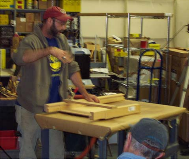
This is a clamping jig Bruce uses to create his rockers for the rocking chairs. Here you can see an actual lamination in the clamp.
