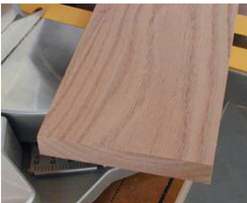
This board was cross cut with a 96-tooth Fine Cross Cut Blade on a Sliding Compound Miter Saw.
